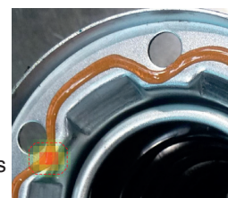
Inspection of a sealing cord
